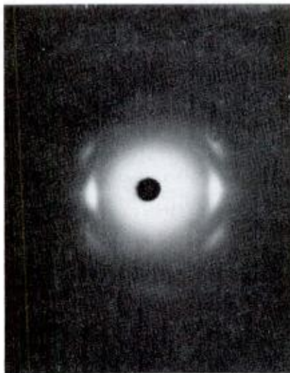
Fig. 3. X-ray diffraction pattern of 5 times-stretched sericin and its schematic representation (Komatsu, 1975)
